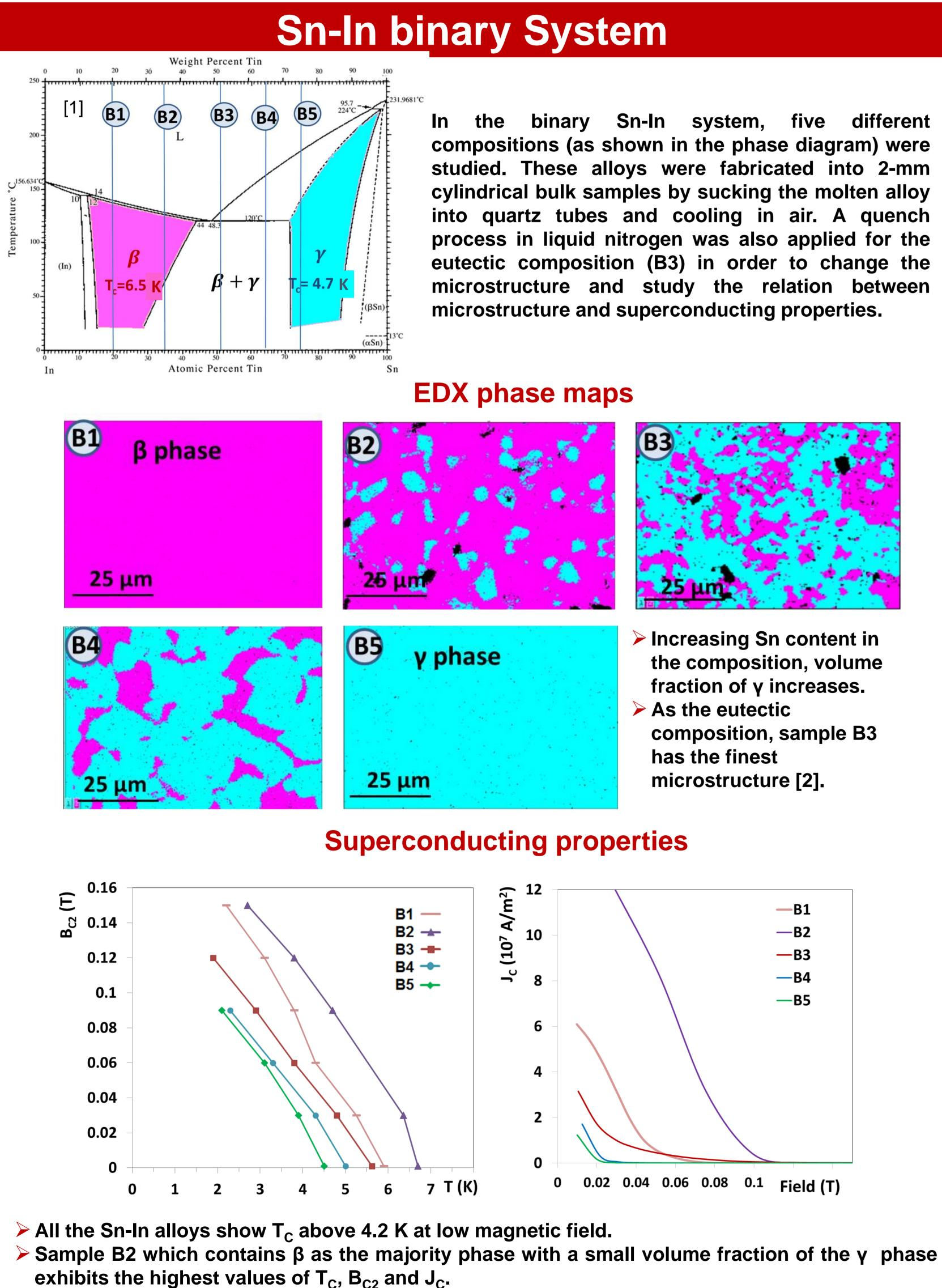
$\blacktriangleright$  Sample B5 which is pure  $\gamma$  phase has the poorest superconducting properties. In two-phase samples, superconducting properties improve by increasing volume fraction of the β phase.
