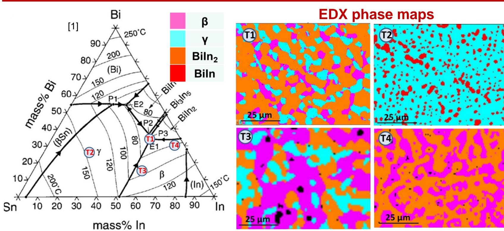
• Four different ternary alloy compositions (T1-T4) were fabricated. EDX phase maps indicate that a variety of microstructures with different phase fractions, chemistry and morphology can be produced.
