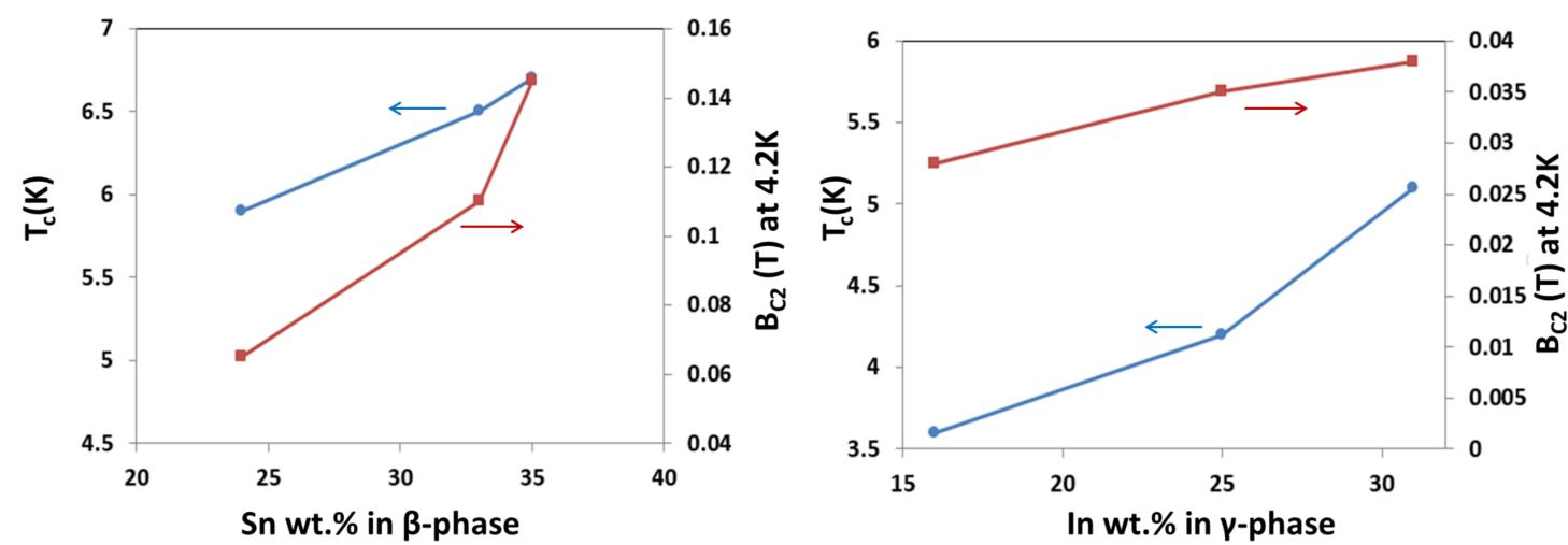
In both  $\beta$  and  $\gamma$  phases, superconducting parameters (T<sub>c</sub> and B<sub>c2</sub>) improve by increasing the solute content. As a result, in the In-rich  $\beta$  phase, increasing Sn content leads to higher values of T<sub>c</sub> and B<sub>C2</sub>, whereas in the Sn-rich γ phase, superconducting properties improve by increasing In content.
